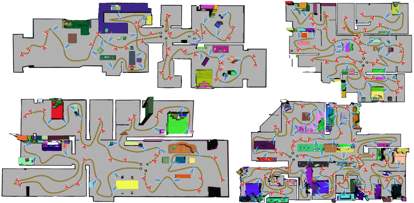
Fig. 10. Some visual results of our method on four virtual scenes (three from the Front3D data and one from the MatterPort3D dataset). The traveling path is represented in yellow lines with black contours, with the exploration tasks (red triangles) and reconstruction tasks (blue triangles) shown on the top of the path.
